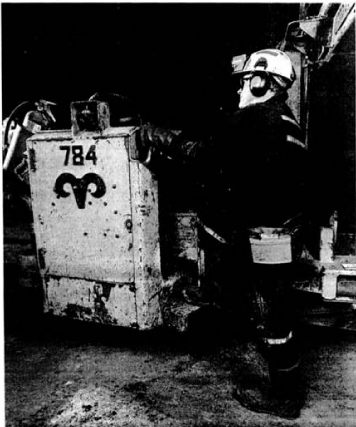
Ergonomics applies to everything. Beyond the work recently done in warehousing, ergonomics has and will continue to help improve safety and production in the Ontario Division. The ergonomic design of handles and steps on this truck work hand-in-hand with safe work practices to prevent injuries. Three-point contact when getting on or off equipment, such as this scissor truck at Crean Hill Mine, is also injury prevention in action as development miner Tom Dolan knows.
