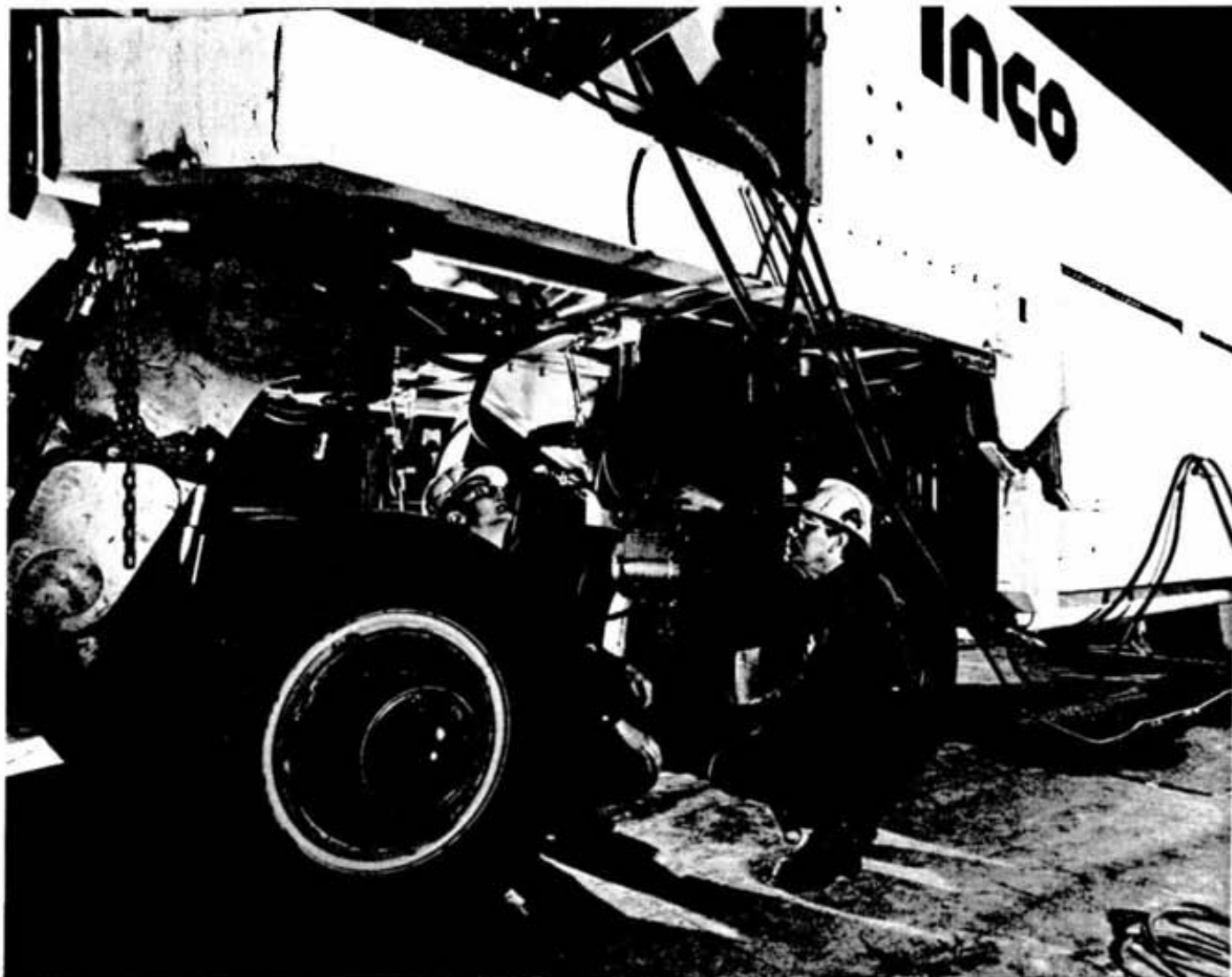
Blair Bennett and Georges Langlois complete the installation of hydraulics on a prototype 70-ton underground electric ore haulage truck.
