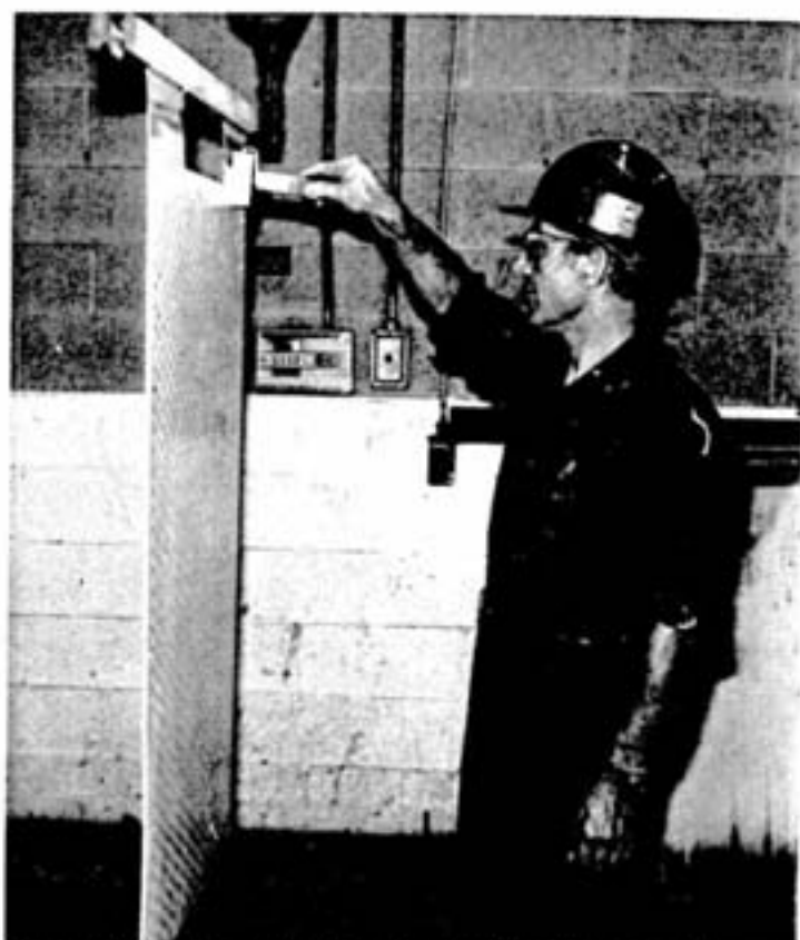
Mario Forte touches up the edges of a sheet after it has passed through an automatic printer. The pattern is applied by a silk screen printing process.
