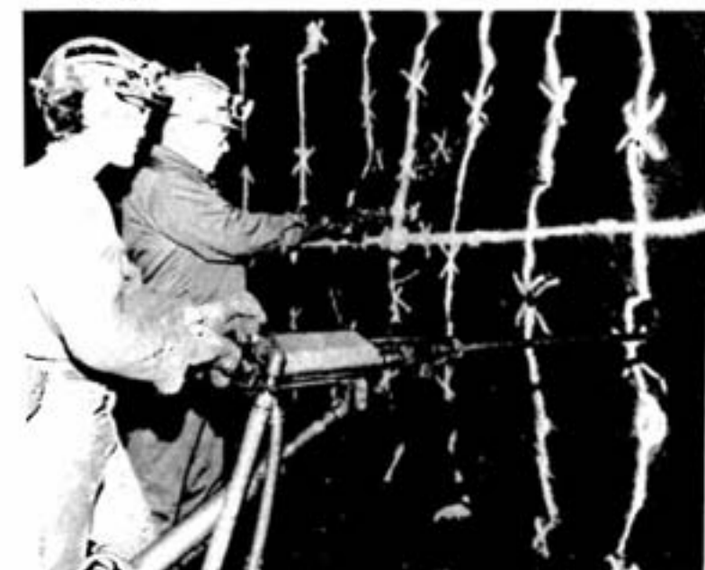
Trainee Rheel Morissette, left, becomes familiar with the jackleg drill, under the careful eye of instructor Armand Ruel. The photograph was taken on the 1800 level of Stobie mine where the mines training area is located.
