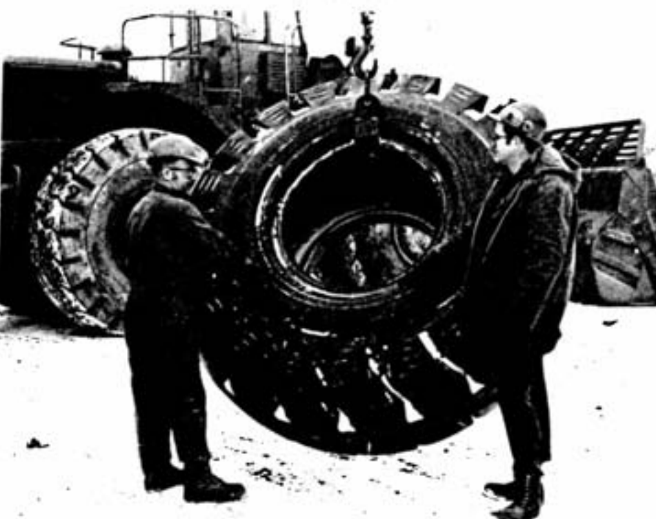
Calder MacLeod , tire serviceman for United Tire, and Dale Clarke , training supervisor, Copper Cliff North mine, are checking out this $4,500 open pit loader tire. Weighing in excess of 3,000 pounds, this 33.25 x 35" monstrosity is only one of the more than 1,700 loader tires in operation at Inco mines in the Sudbury district. Individual brand numbers are assigned to each tire in circulation.
