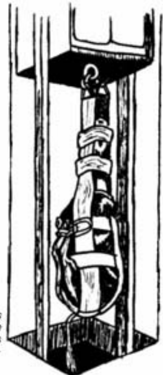
6. The holding hook was built so as to place the mule diagonal in the shaft compartment. This was necessary due to the small compartment size.
