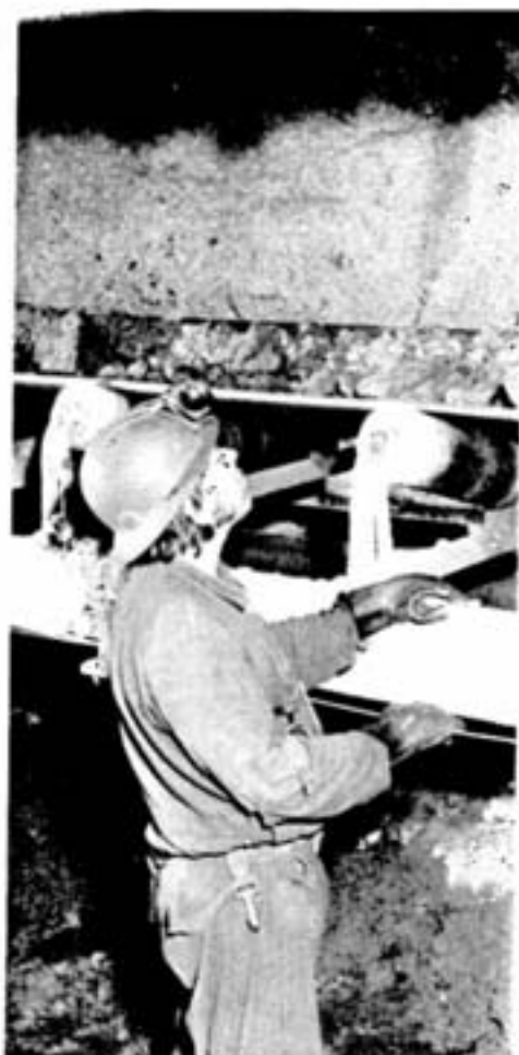
Dennis St. Martin inspects the main ore conveyor on the 1950 level. This conveyor carries the partially dried sludge to the shaft where it's hoisted to surface.
