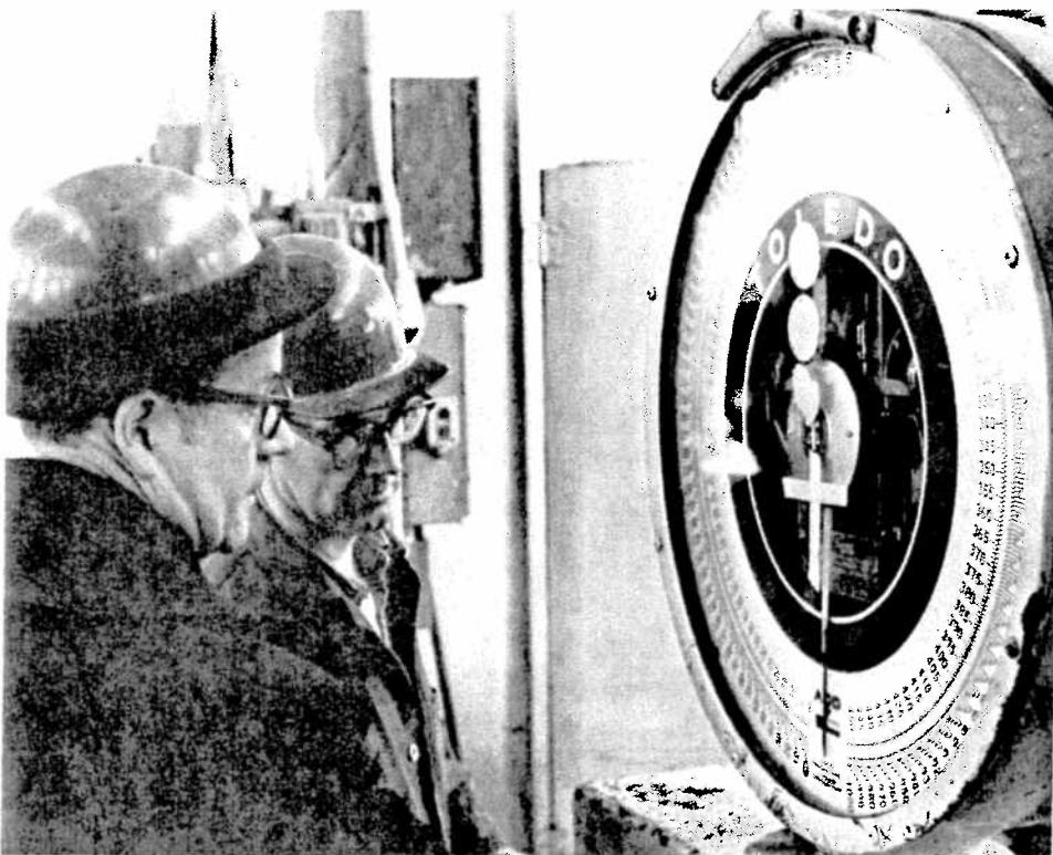
Elvin Bearss and Stew Rowland confer about one of the shearing department's half-ton dial scales. Minor accidents, such as falling boxes, often destroy the scale's balance.
